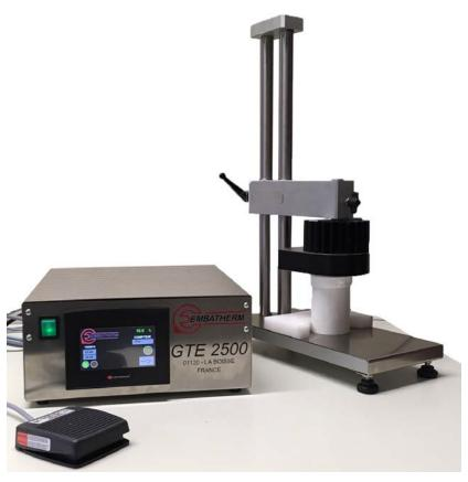
This machine is designed to seal heatseal aluminium based liners through the caps onto plastic or glass containers.
