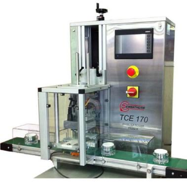
The operator places the jar on the conveyor. Some sensors detect the jars and trigger the sealing operations. Holding, pre-cut seals adjusting on jars and sealing are made in a single operation. The sealing as well as the centering of the seal are perfectly repeatable. Then, the sealed jars are evacuated toward, either an operator in charge of capping the jars, or an accumulation table.
