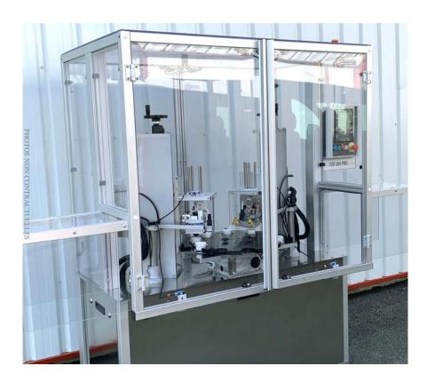
These machines are designed for the automatic heat sealing of pre-cut lids on all types of rigid plastic or glass packaging (treated for ideal sealing) and are intended to be inserted on the main conveyor of your packaging line.
