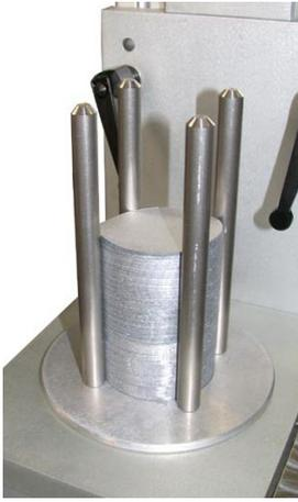
These heads ensures the hold, the set and the heatsealing of the aluminium pre-cut foils in a single operation. The pre-cut foils stacks are set in trays that are interchangeable and refillable without stopping the machine.
