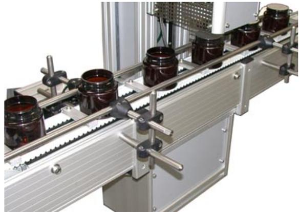
Whatever the machine version, every parameters are user-definable and displayed (time, pressure, temperature or power of sealing) on the tactile screen, as well as the working state of the machine and potential defects.
